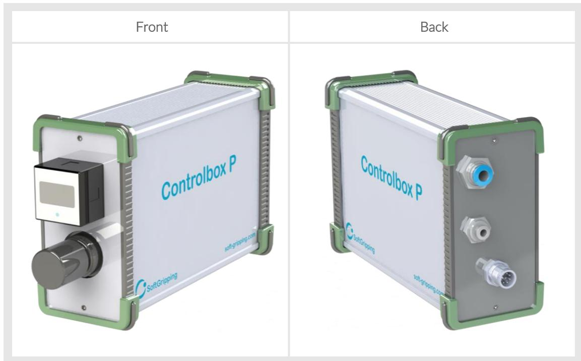
The control box is used to operate any SoftGripper or End of Arm Tooling. On the front, the current pressure can be seen in the pressure indicator and adjusted via knob. On the backside of the device you can find the pressure input and output. The output is controlling the position of the fingers. You can switch between 2 positions: Grip and Relaxed setting the according Signal Connector's pin to high (Grip) or low (Relaxed).
